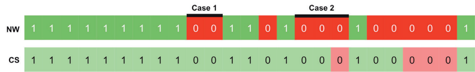
Fig. 3: Comparison of network (NW) and communication service (CS) failures depending on the survival time
