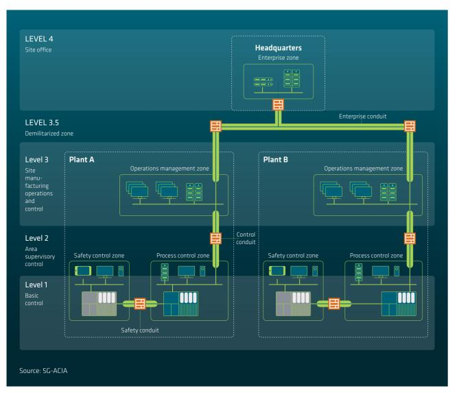
Each zone can be treated as a separate network slice, i.e. headquarters, plant A and plant B would be separate slices with slice-specific authentication (on top of primary authentication). This provides logical separation between the member groups. The conduits can be implemented by means of WAN connections. Based on the security level of each zone, core network functions might have to be implemented separately for each slice.
