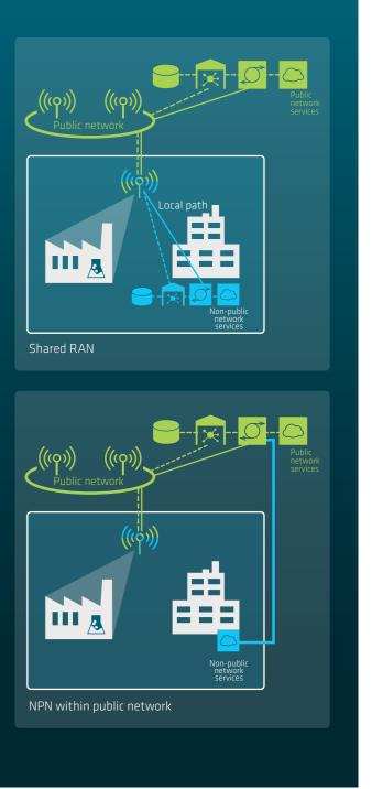
network. This scenario would significantly benefit from 5G network slicing features for its implementation. 5G closed access group (CAG) functionality can be used for access control in this scenario [5].
