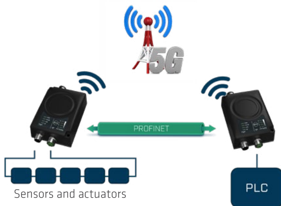
Figure 20: 5G Ethernet bridge in a typical cable replacement use case (source: HMS Networks)
