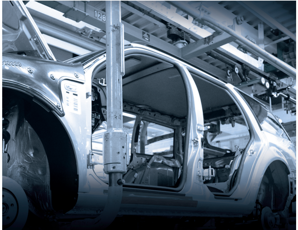
Fig. 2: Body-chassis marriage in automobile manufacturing
